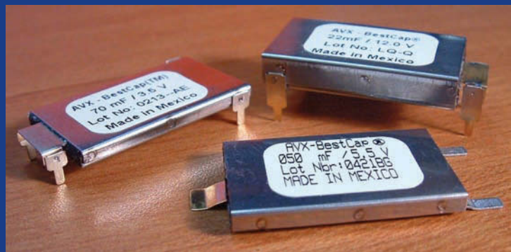
Figure A AVX supplies EDLCs in a variety of cases, including these 28×17-mm units. The case thickness depends on the energy a device can store. You can calculate the stored energy using the formula W = 0.5 \times C \times V^2 , where W is the stored energy in joules, C is the capacitance in farads, and V is the working voltage in volts. Clockwise from left, the values are 0.429, 1.584, and 0.756J.
